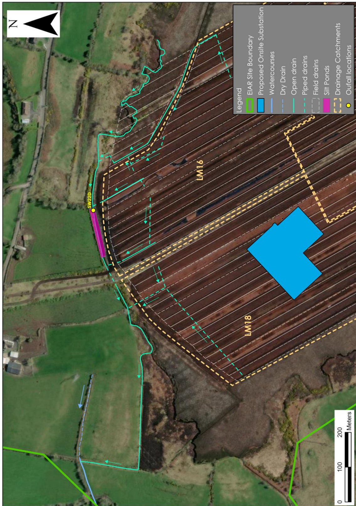
Figure I: Existing Drainage at the Proposed Onsite 220kV Substation Area
